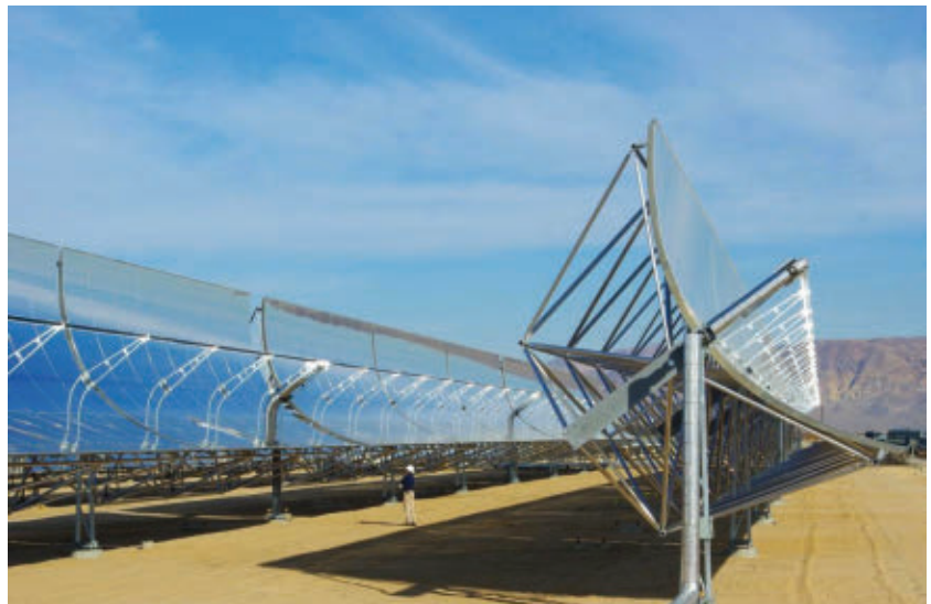
SkyFuel’s parabolic trough concentrating solar collector. Credit SkyFuel.
