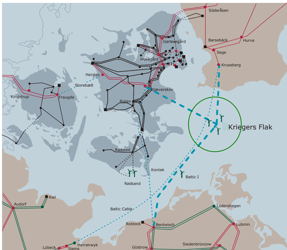
Figure 1 Location and sketched connection of Kriegers Flak. The thinner dashed lines indicate the existing connections between Denmark and Germany (Kontek) and Sweden and Germany (Baltic Cable). Source: Energinet.dk
