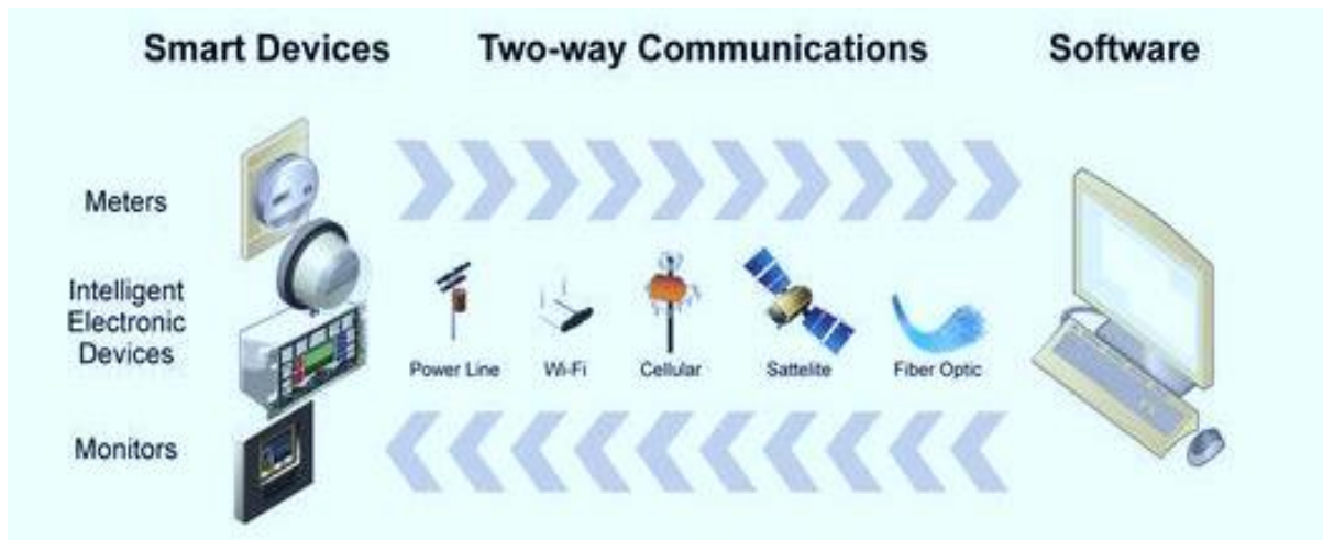
Figure 11: Smart Grids Provide Two-way Communication
