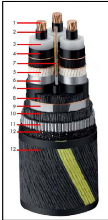
Fig 16: Modern Submarine Power Cable (AC)
