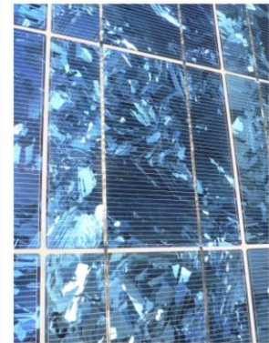
Figure 26 Silicon-Solar-cell in a solar module Source: http://upload.wikimedia.org/wikipedia/commons/1/15/Polycrystalline-silicon-wafer_20060626_568.jpg
