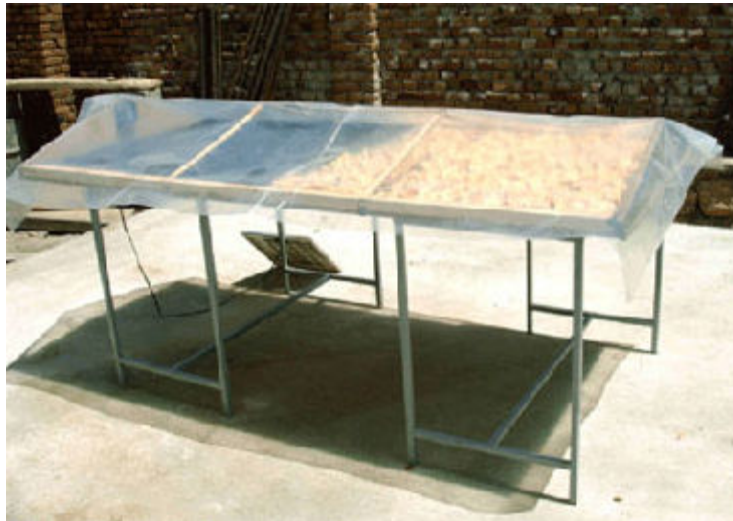
Solar tunnel dryer, 2m x 1m
