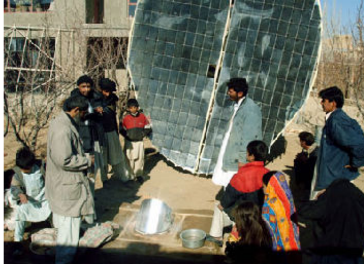
Scheffler Reflector at the Center for Renewable Energy in Bedmoschk. A traditional Tandoor oven is heated with solar power.
