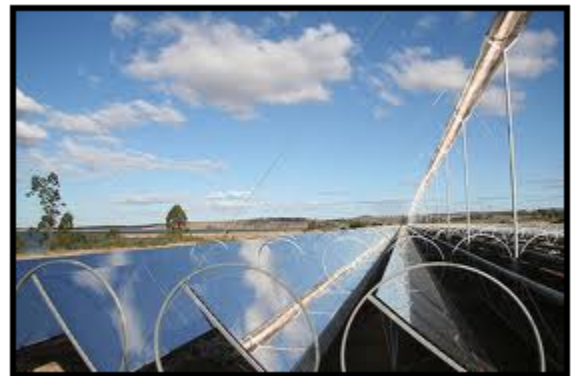
Figure 13: Linear Fresnel Reflector (Ausra)
